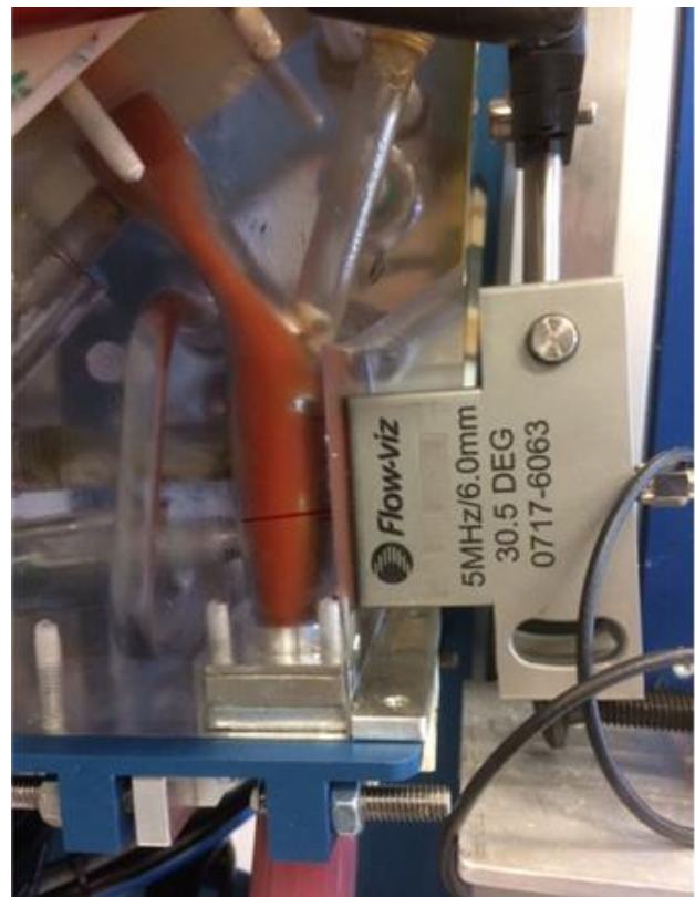
Figure 2: Photo of the customized UVP sensor measuring the flow of ketchup inside the pharynx.
