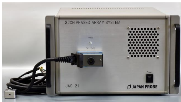
Figure 2: Photograph of 32ch pulser/receiver and array sensor.
